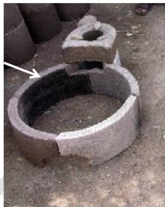
Figure 2: Mirt stove with baking plate (“mitad”) and cover 4 and slim Mirt without baking plate 5
